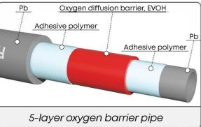
Oxygen barrier PB pipes have a layer of polymer laminated to the outside surface (or sandwiched internally between PB layers) that prevents oxygen from penetrating. The polymer film is usually EVOH (ethyl vinyl alcohol copolymer), used in the food industry as an oxygen barrier.
